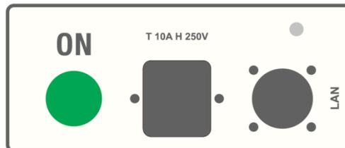
The Ethernet port of the Erigo PC is configured to use DHCP by default and should therefore be compatible with most existing computer networks.
